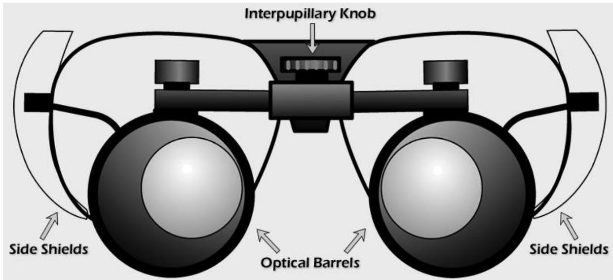
The components of the loupes as shown. The *Interpupillary Knob* adjusts the lateral distance from one barrel to the other. This should be the **ONLY** adjustment you will need to make. This knob does not need to be adjusted each time you use your loupes. Once set properly, it will not need readjustment.
